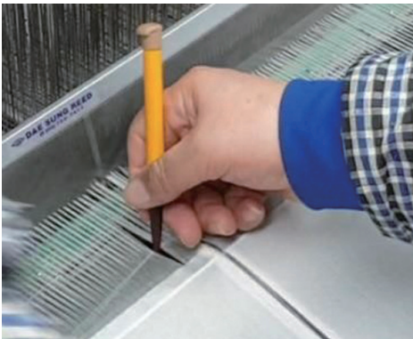
Figure 19. Heumdae is used to unweave the weft yarn (photo by author, 2021).
