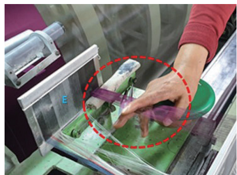
Figure 14. Winding after identifying the yarn tension (photo by author, 2021) ( left ).
