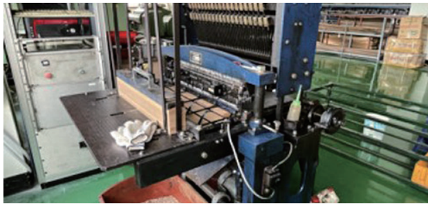
Figure 7. Jacquard card punching machine (photo by author, 2021).
