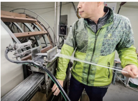
Figure 14. Winding after identifying the yarn tension (photo by author, 2021) ( left ).
